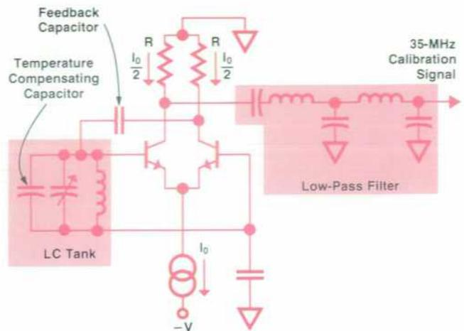
The tank circuit for the second local oscillator includes two parallel varactors that enable the oscillator frequency to be switched from 2.6861 to 2.6711 GHz for the alternate IF.
