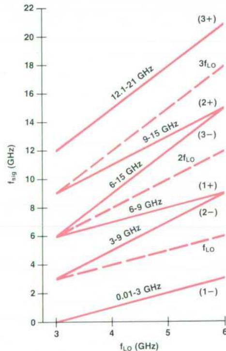
**Fig. 5.** Tuning curves for the 8559A Spectrum Analyzer. The numbers in parentheses adjacent to each range indicate the harmonic used to obtain a 3-GHz IF for that range. The analyzer's SIG IDENT pushbutton helps the user identify the proper range for a particular signal.
