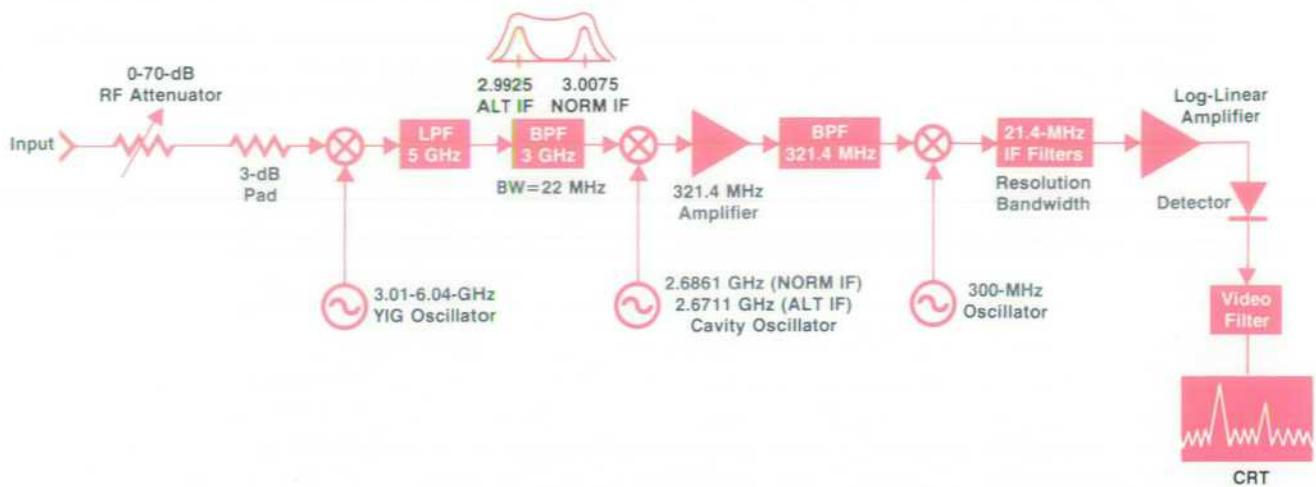
**Fig. 4.** Simplified block diagram of the Model 8559A Spectrum Analyzer. Except for the alternate IF scheme, it follows conventional practice. The input frequency is converted to the 21.4-MHz final IF in three steps to allow adequate frequency separation between the desired signal and its image at each conversion.
