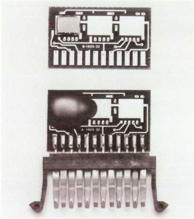
**Fig. 3.** ROM modules contain one or two chips, each measuring 3.71 by 5.00 mm and containing 40K bits. The bit pattern is customized for each application. There are 7-9 bonds per chip and ten connections via a reflow-soldered contact frame to the HP-41C. The substrate measures 23.37 x 13.72 x 0.79 mm.
