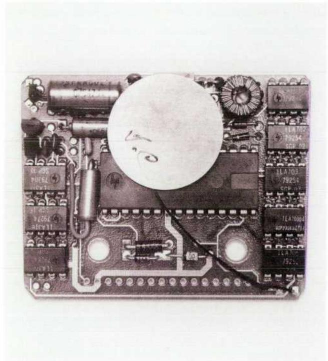
Fig. 2. HP-41C logic board.
