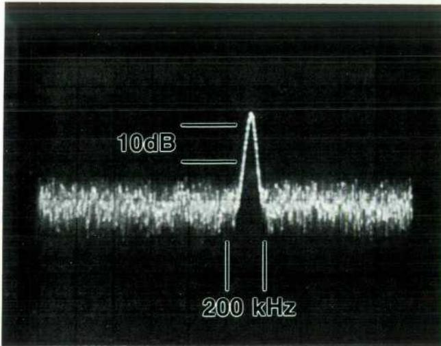
**Fig. 2.** An example of the 8559A's lab-grade performance is this display of a  $-57$  dBm signal at 20.39 GHz. The resolution bandwidth used was 30 kHz and the noise level is  $-83$  dBm. This corresponds to an average noise level of  $-98$  dBm in a 1-kHz bandwidth (specified maximum is  $-90$  dBm).
